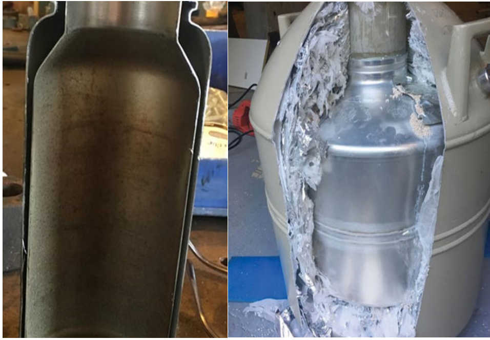
Figure 2: A commercial Thermos flask (left) and a liquid nitrogen Dewar (right) cut into sections. The MLI made by hundreds of aluminized Mylar foils as well as the composite neck are visible.
